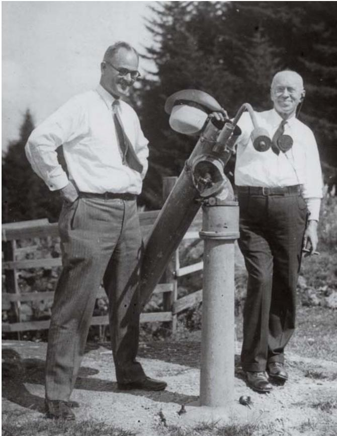
▲ **STARS** Albert G. Ingalls (left) and Russell W. Porter pose in the early 1930s with a reflector on an equatorial “Springfield mount” of Porter’s design. It kept the eyepiece at a fixed position, at the cost of three mirror reflections and a high counterweight.
