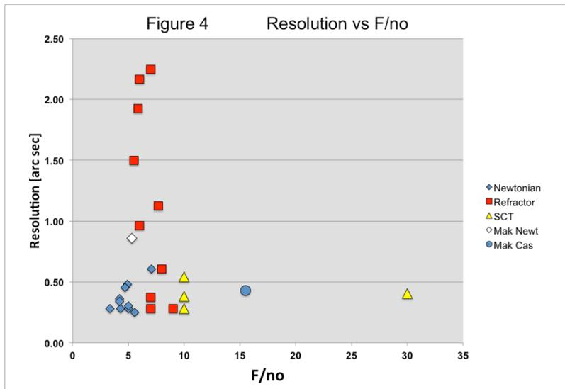
achieved is shown in figure 4. This plot clearly highlights the limited range of f/numbers for each telescope type, but does not show any other clear correlation.
