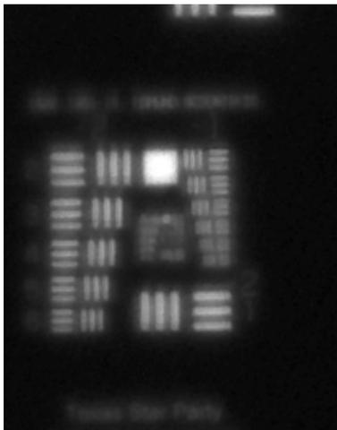
SCT with a x3 barlow operating at f30 and a video camera for image capture. Using the “lucky imaging” technique he captured many two thousand frames, selected the best 100, and then aligned, stacked and sharpened the result using Registax 6. An example resulting image is shown here.
