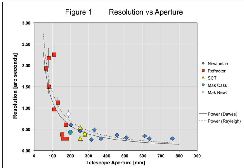
the telescopes all failed to reach the Dawes limit and we may possibly attribute this to poor seeing (see later section), and their inherent general design of being fast f/no light collectors with less than diffraction limited performance other than exactly on-axis.
